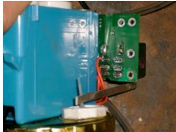
**Cover All active relay lugs with RTV for insulation (red wires) to preclude shock hazard. Mount PC board to the blue box using 2 ea. #4 sheet metal screws and a two high stack of washers between the PC board and the blue box.**
