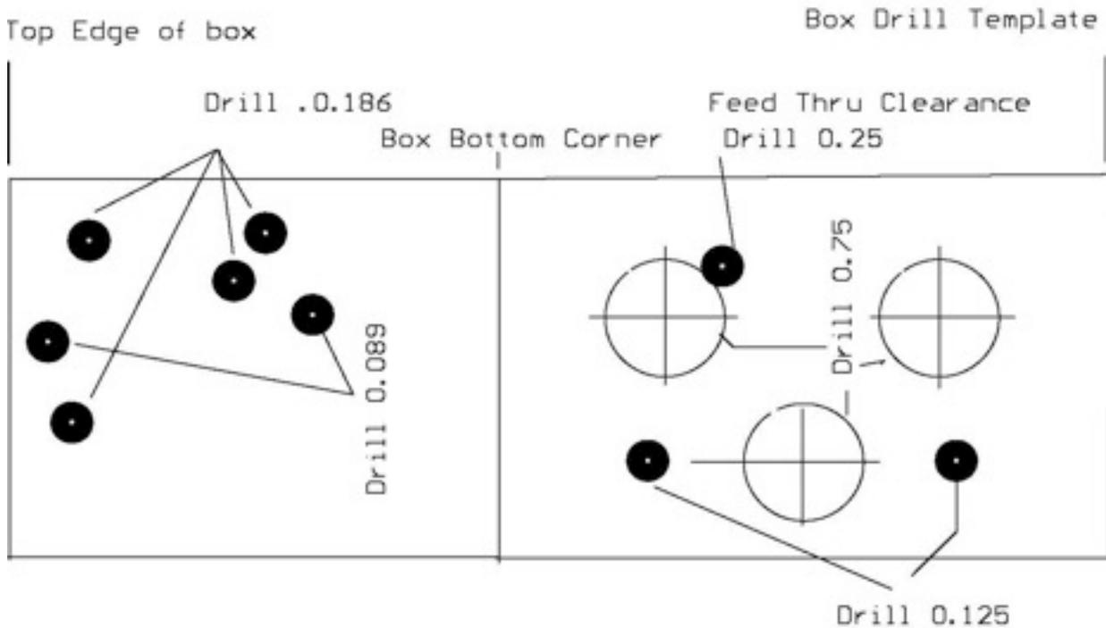
Blue box drill template cut off the box nail mount tabs fold template around box
