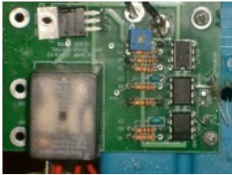
**Dryer control electronics board**
