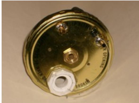
**Drilled lid with paint removed at brass tube solder locations**
