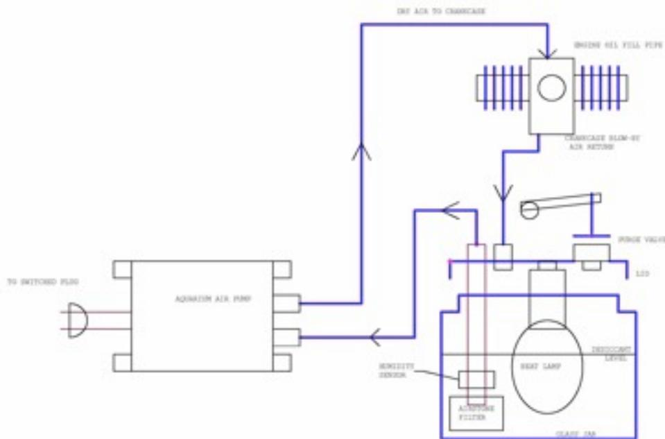
Mount the lamp socket to the lid and secure with the hollow mounting bolt.
