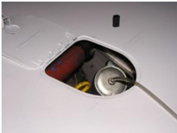
**Engine air input fitting to oil filler cap
