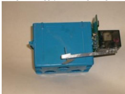
Purge valve control pc board mount on electrical outlet box
