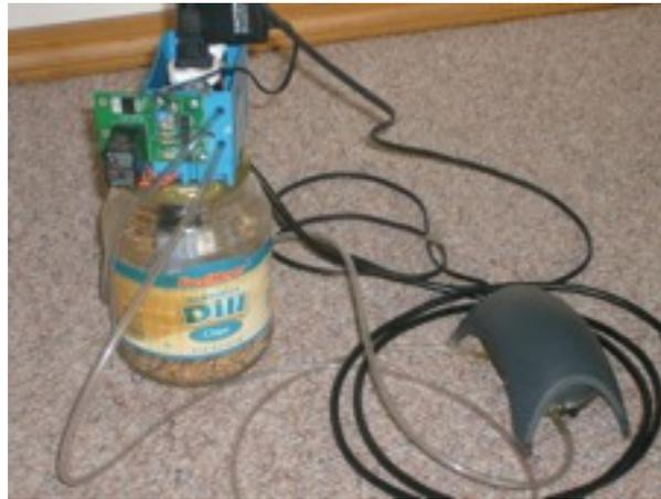
Automatic Purge Engine dryer and pump
