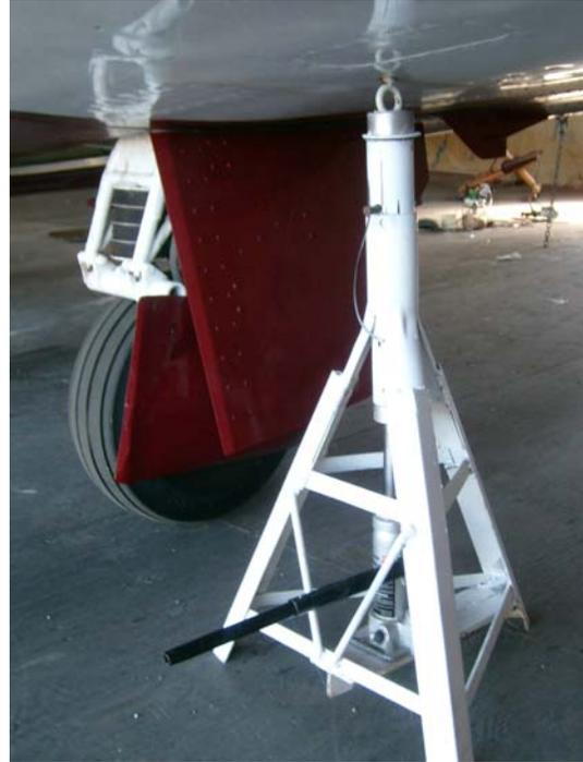
The two jackstand frame extensions will require 6 pieces of 1" x 1" x 1/8" steel angle iron cut to ~18" in length. One end of each piece will need to be bevel cut (both faces) at ~ 65° (to the vertical) or 25° (to the floor) in order to sit flush on the floor. Clamp and tack weld one leg on to the jackstand. Attach the other two legs with C clamps and adjust the leg lengths to make the axis of the jackstand vertical before welding the other legs.
