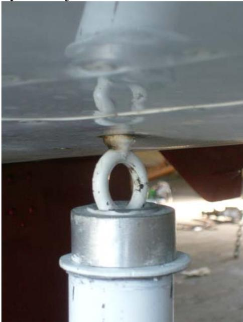
Determine the maximum available height between the wing jack point and the floor. Set the leg length to easily slide the stand under the wing and clear the jack point.
