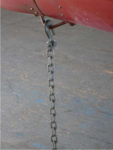
However, many aircraft service shops employ a large weight in the form of a wooden box filled with concrete and mounted on casters for ease of movement. A chain or vertical pipe and locking pin cast into the cement is used to anchor the tail in position. This weight may have to be on the order of several hundred pounds depending on the aircraft type. That part of the project is left to the innovation of the reader.
