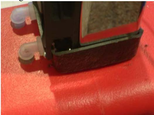
**ABS L bracket mount goes inside fan flange and over the front lip of the radiator.**
