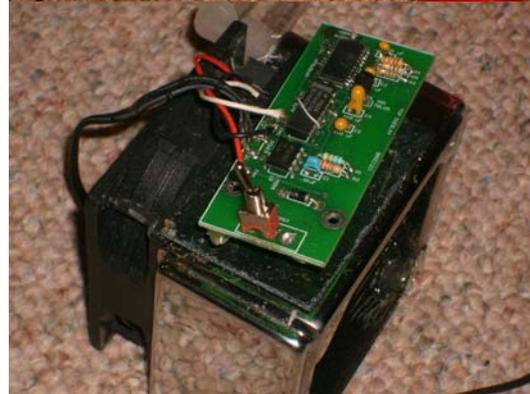
Position and glue the ABS 2x4" sheet on top of the radiator. Note: Switch mounts in rear two holes .
