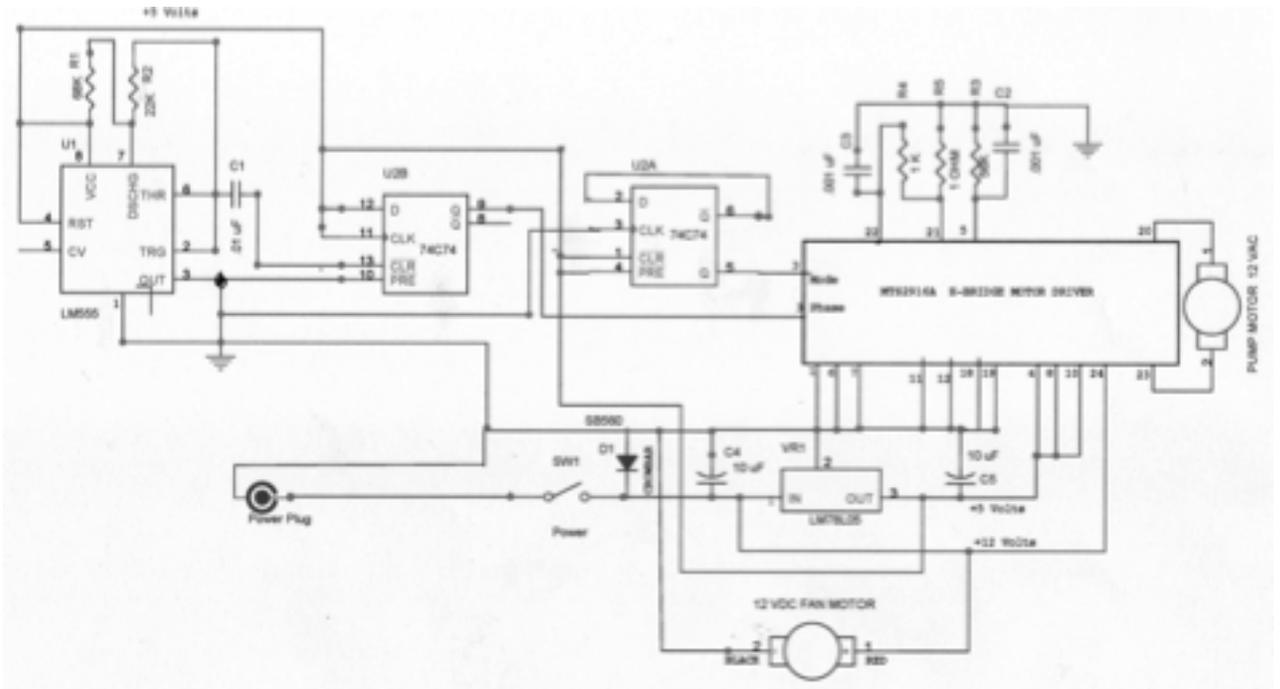
to generate a symmetrical 60 Hz square wave. The MTS2916A is a single chip stepper motor controller and
